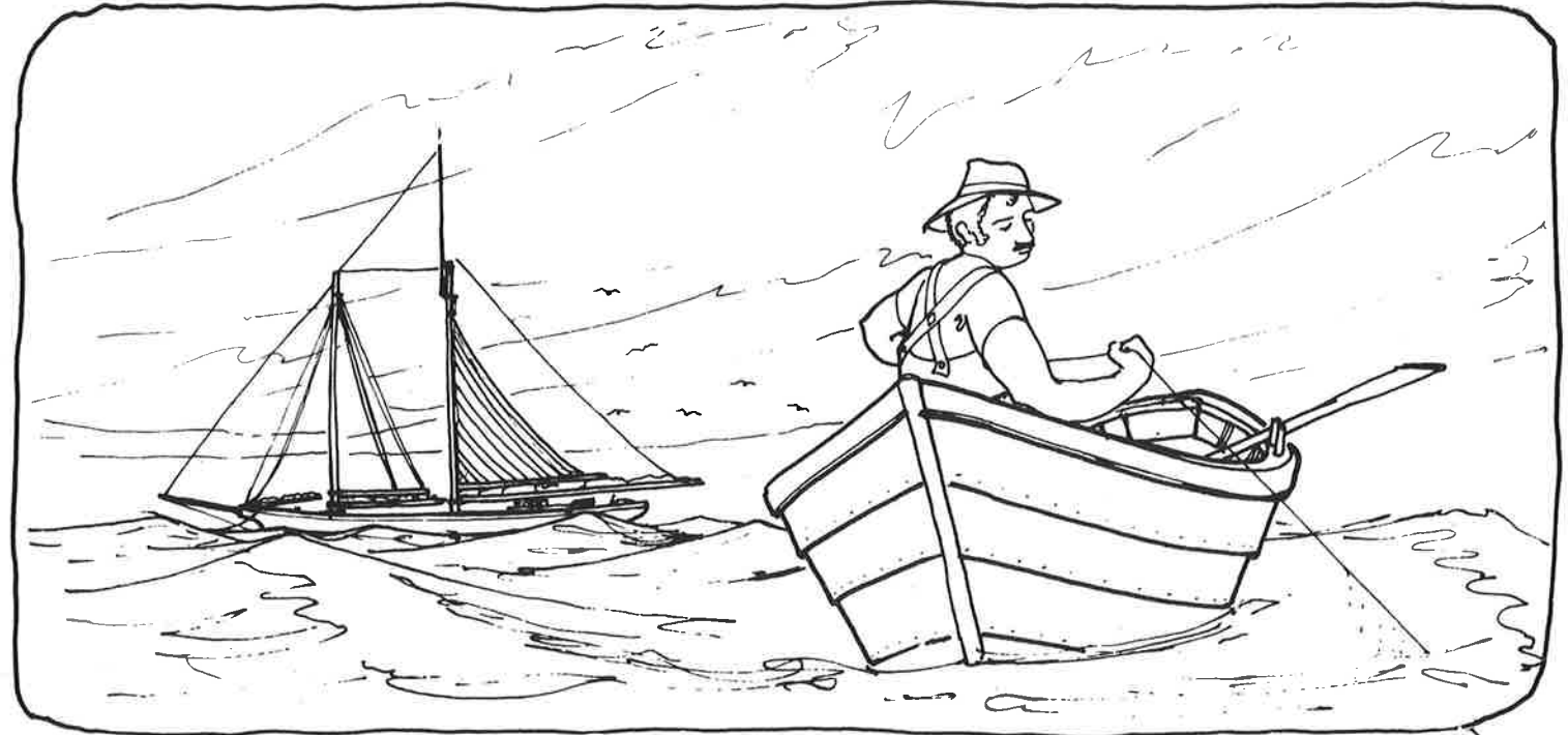
THE LETTIE G. HOWARD AT WORK, ANCHORED ON THE BANKS (SHALLOW PARTS OF THE SEA WHERE FISH LIVE). A CREWMAN FISHES FOR COD WITH A LONG LINE. WHEN HIS DORY IS FULL, HE WILL ROW BACK TO THE HOWARD, UNLOAD HIS CATCH, AND GO OUT AGAIN. IF THE SCHOOL OF FISH MOVES AWAY, THE HOWARD MUST RAISE ANCHOR AND FIND ANOTHER SCHOOL.
