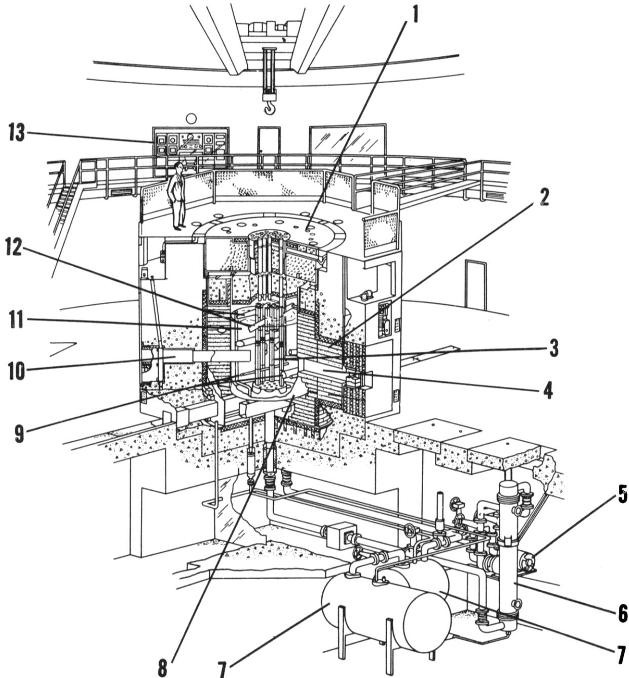
FIGURE 36.—Argonne Research Reactor (CP-5) Tank Type with Heavy Water, (1) Access to Vertical Thimbles, (2) Graphite, (3) Fuel Assemblies, (4) Thermal Column, (5) Circulating Pump, (6)  $D_2O-H_2O$  Heat Exchanger, (7)  $D_2O$  Storage, (8) Reactor Tank, (9) Pneumatic Tubes, (10) Beam Hole, (11) Heavy Water ( $D_2O$ ), (12) Control Arms, and (13) Control Room.
